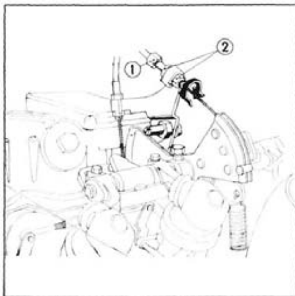
Fig. 20-20 Throttle cable adjustment
