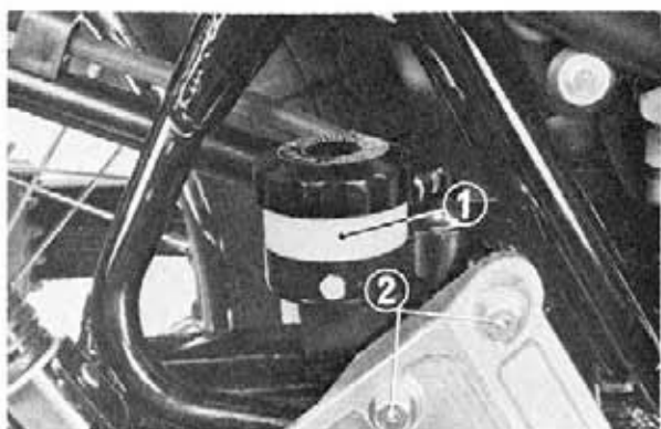
Fig. 26 ① Master cylinder
