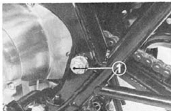
Fig. 15 ① Rear fork pivot bolt
